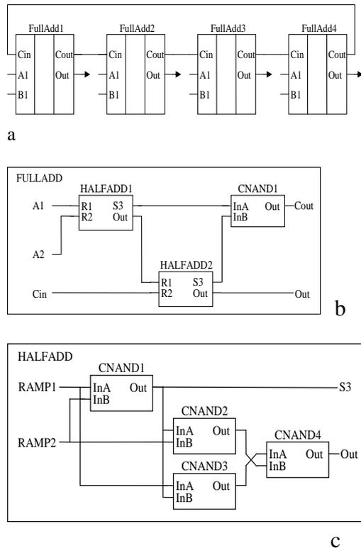
Pic. 1. Test circuit *FADD32*: a – its structure; b –subcirciut *FULLADD*; c – subcirciut *HALFADD*.
